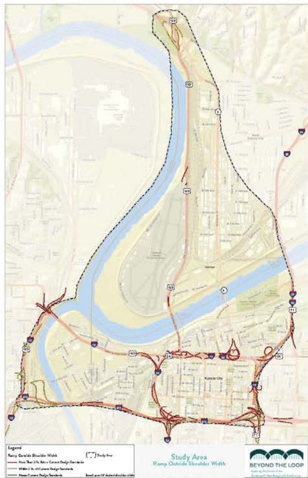
Figure 2.7 - Outside Ramp Shoulder Widths
