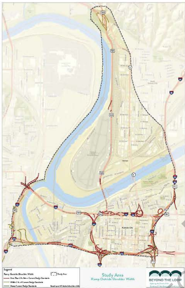
Figure 2.7 - Outside Ramp Shoulder Widths
